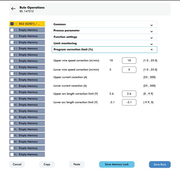
You can influence the welding quality and manage welder by editing the maximum and minimum values for the wire speed, current, and voltage set on the machine to restrict the machine within a defined maximum and minimum range according to the set values.
