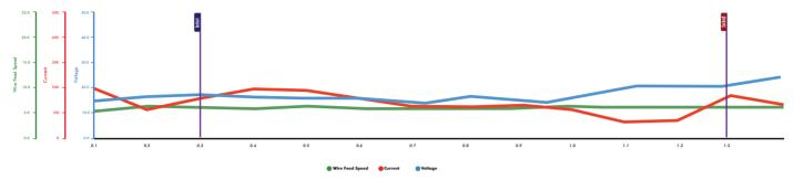
Data graph generated with real-time wire speed, current, and voltage values at 100 ms intervals during welding.
