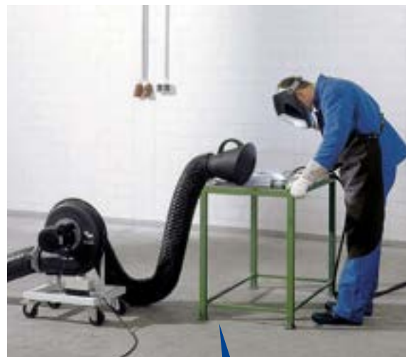
Example of application: Mobile exhaust fan
