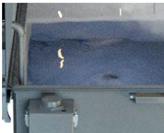
The sparks drop into the water and extinguish
