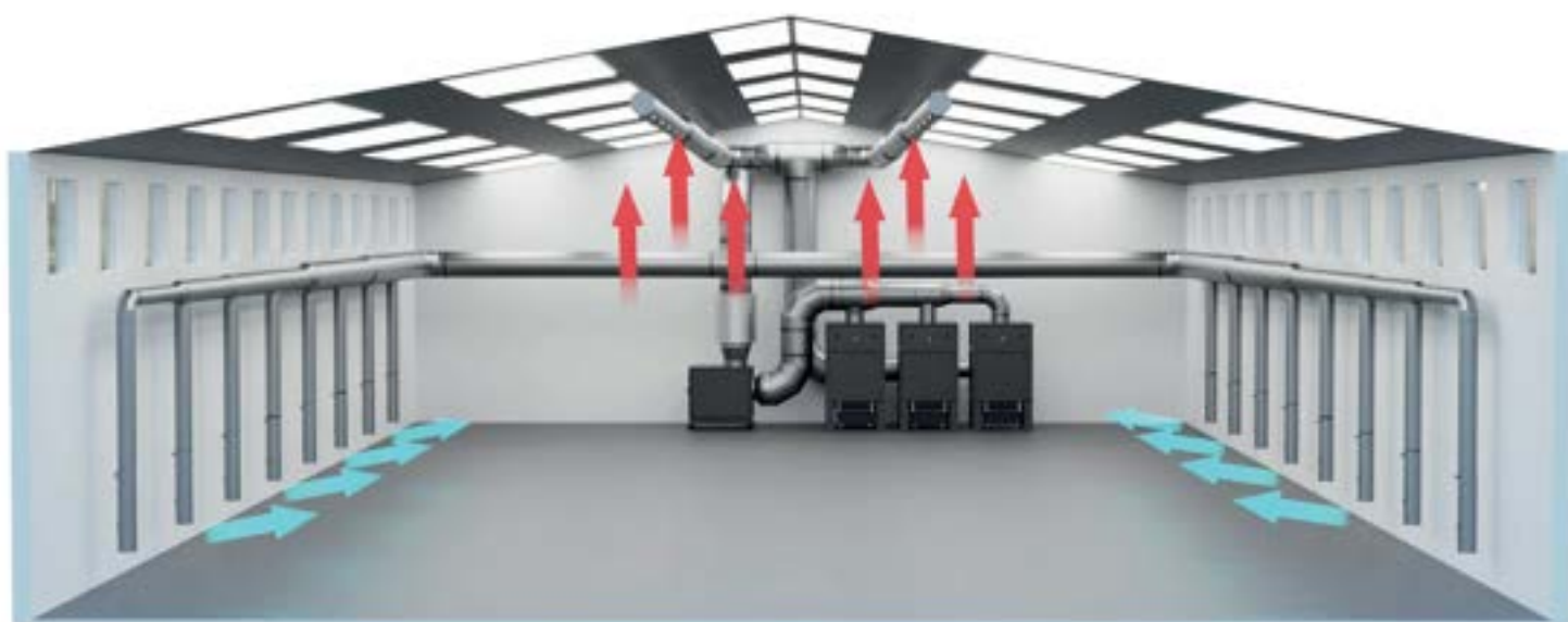
Installation example: Layered ventilation system in a hall
